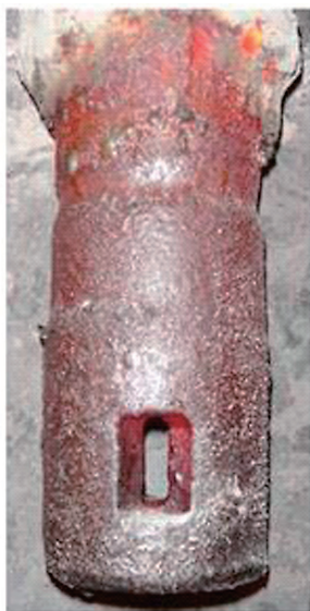
Fig.14 Appearance of "Bend port" SEN after use and comparison of the bleeding defect rate.
